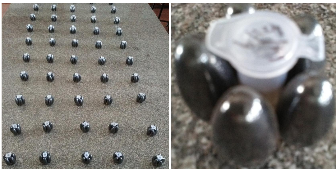
Figure 2.1 Precursor iron molecular solutions kept in the magnetic field for the synthesis of SPIONs
