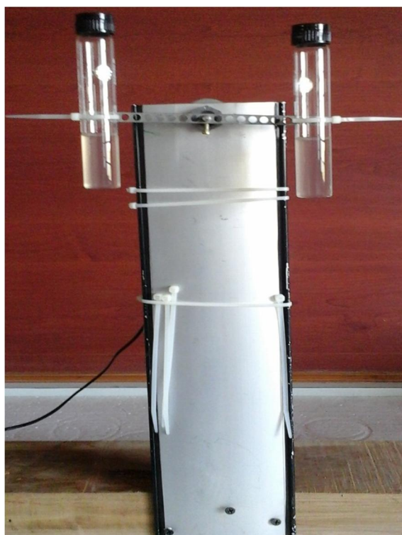
Figure 2.2 Cyclo rotator designed to give specific agitation during functionalization, drug loading and encapsulation
